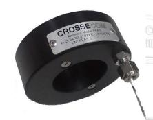
The antenna, mounted conveniently on the dispensing nozzle spout, comprises a small loop antenna with its low power electronic components. It is connected to the reader (mounted inside the pump housing) via a special petroleum resistant cable.
